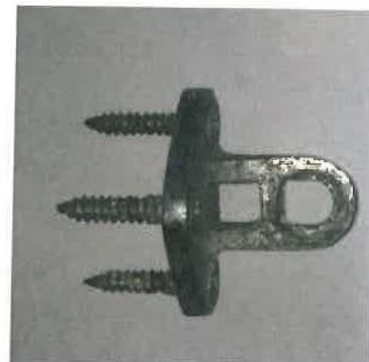
one inch wood screws used to secure the brackets for the hatch cover.
